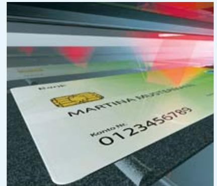
When the card is inserted into a cash machine, the reader scans the surface in detail. The laser strikes the film at an oblique angle, detecting the tiny metallic particles it contains.
